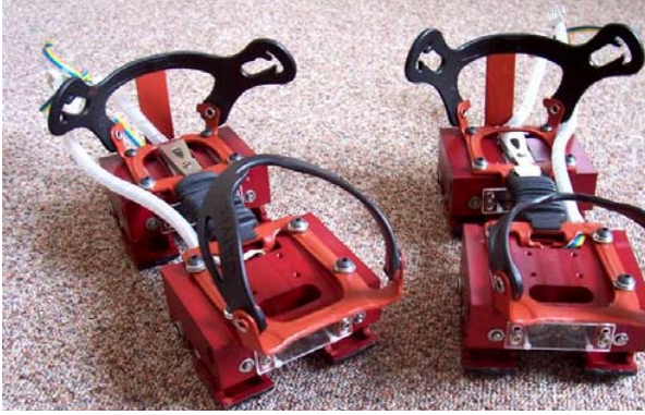
Fig. 1. Completed anodized motorised shoes. The umbilical cords hold the electrical leads
