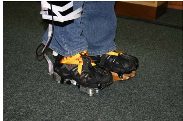
Fig. 15. SMILING shoes with jack-screw TUKE testing mechanics
