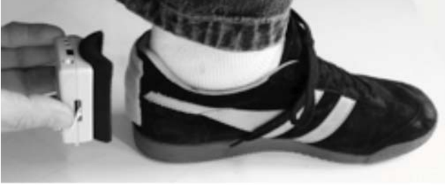
Fig. 1. Foot-worn sensors module (S-Sense) with compliant foam attached to shoe.
